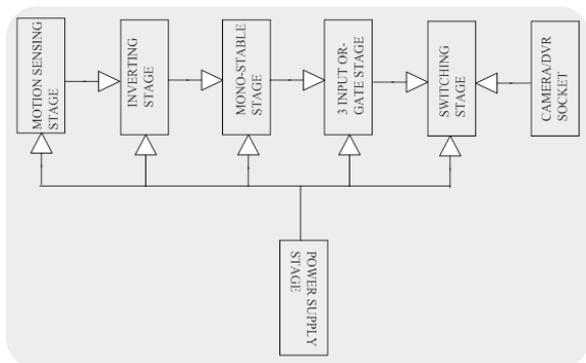
Fig 3. Block diagram of stages involve in the system
