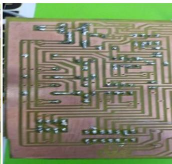
Fig 7. Soldering the components on the PCB
