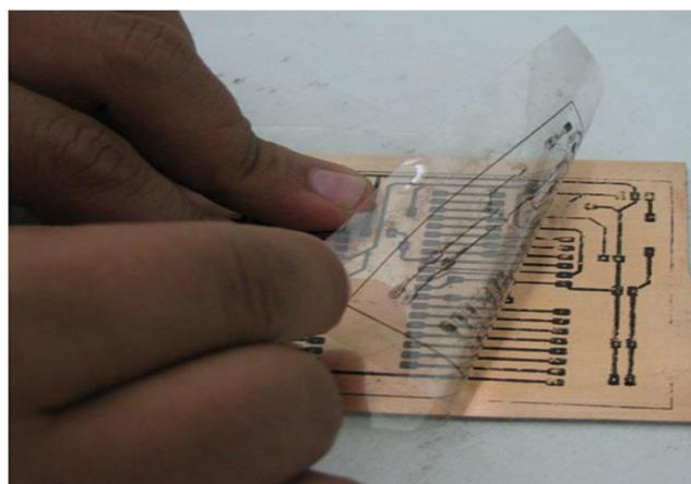
Fig 5. Opening of the Ironing on the PCB
