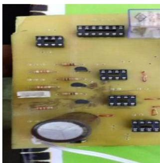
Fig 6. Fixing the components on the PCB
