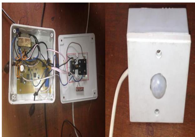
Fig 8: Control system and PIR Sensor
